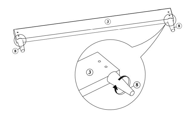
STEP 4: Attach (3) to (4) and (5) Using a Allen Key M5 (B) as shown
