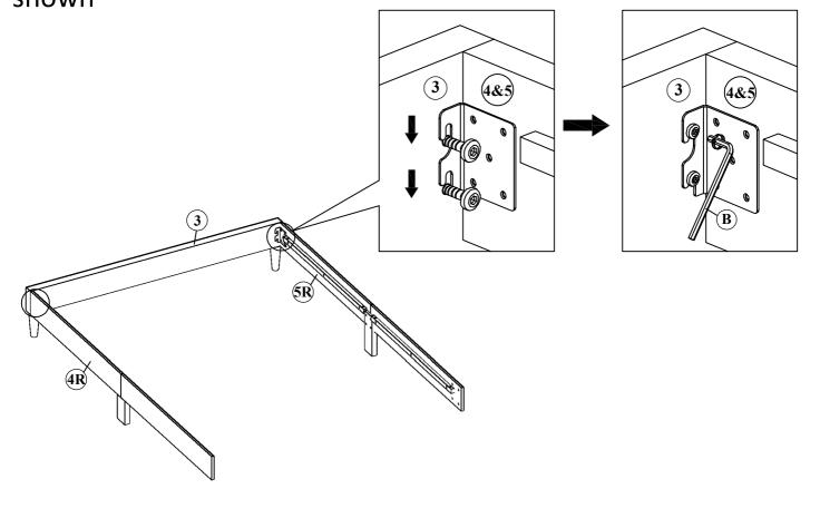
STEP 5: Attach (4) and (5) to (2) With (E),(H) and (I) Using a Allen Key M4 (A) as shown.
