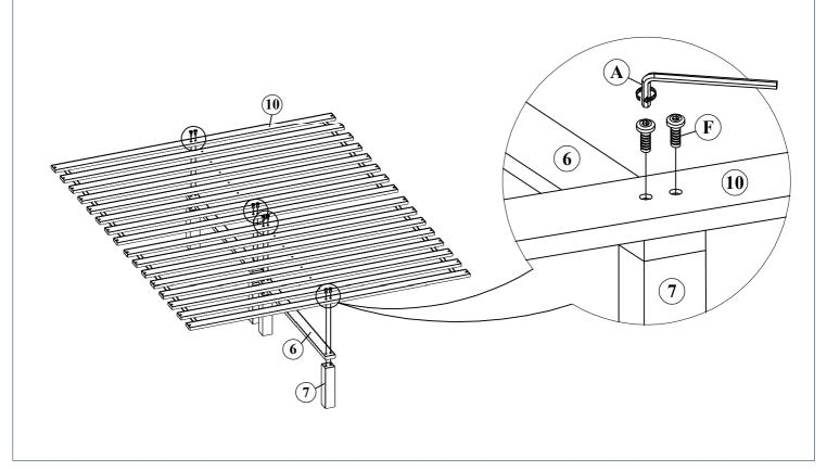
STEP 7: Attach Assembled Bed Slats to Assembled Bed Frame with (C) Using a Allen Key M4 (A) as shown.
