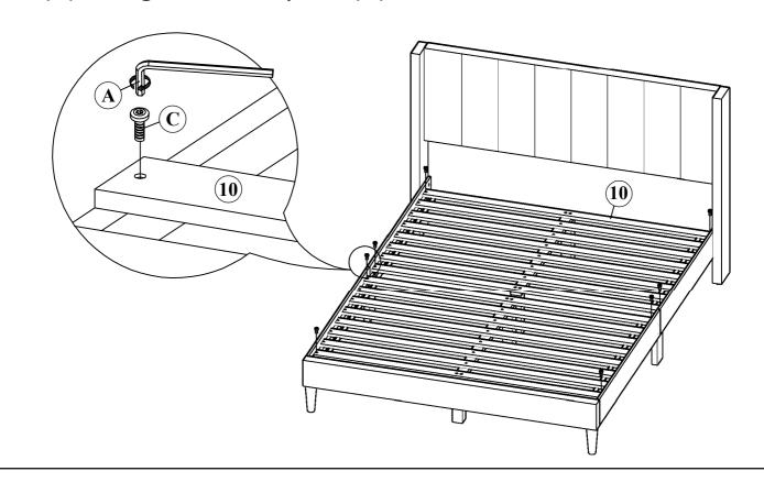
STEP 8: Attach Assembled Bed Slats to Assembled Bed Frame with (G) using a Screwdriver as shown.
